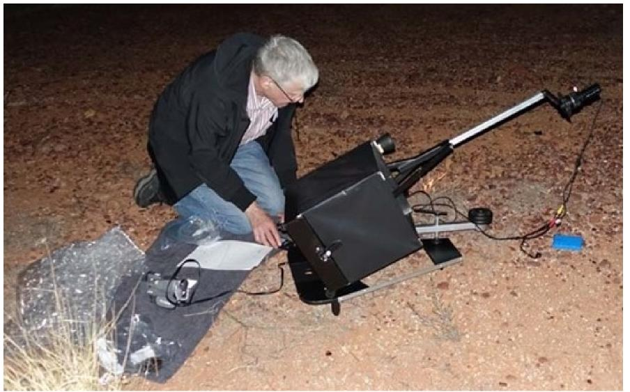
The camera is at prime focus, so the images are reversed (one reflection); it is normally used for pre-pointed occultations of faint stars by asteroids (built by John Broughton).
